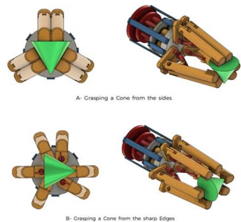
Figure 13. A – Grasping a Cone from the sides. B – Grasping a Cone from the sharp Edges
