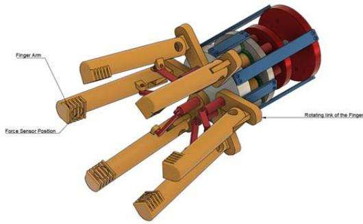
Figure 1. New Modular Gripper Assembly
