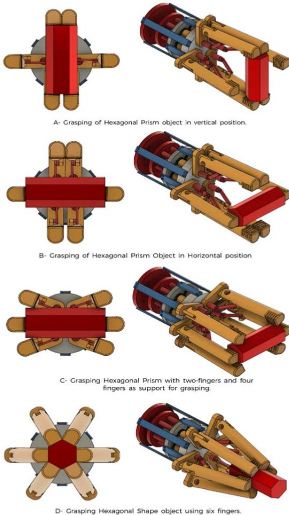
Figure 17. Grasping of Hexagonal shape objects in three different finger configurations.
