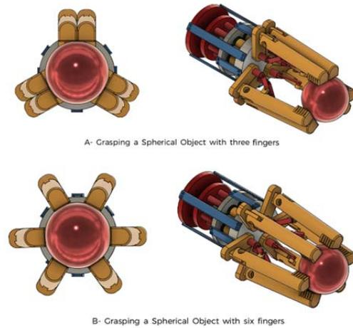
Figure 12. A- Grasping a Spherical Object with three fingers. B- Grasping a Spherical Object with six Fingers
