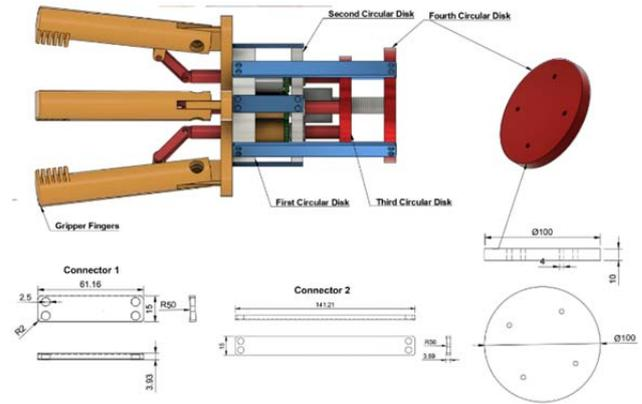
Figure 8. The fourth circular disk and the connectors
