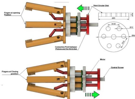
Figure 7. The third circular disk and the movement of the fingers
