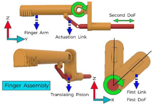
Figure 3. Finger Assembly and the two degrees of freedom
