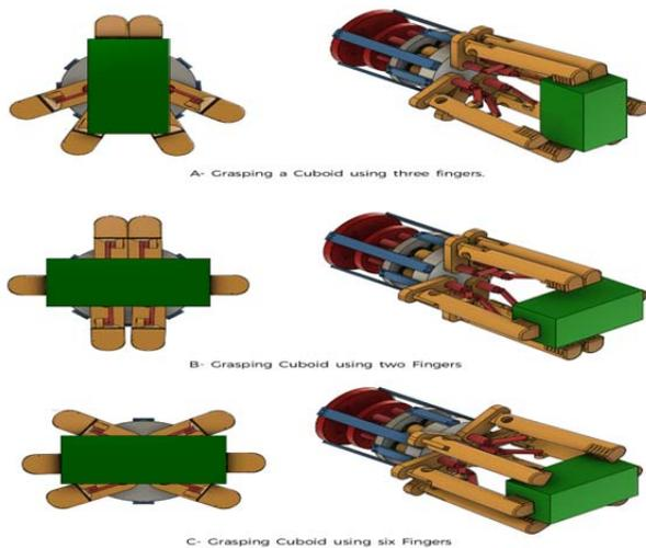
Figure 14. Grasping Cuboid shape object: (A)- Grasping Cuboid using Three-Fingers. (B) – Grasping Cuboid using two Fingers. (C)- Grasping Cuboid using six Fingers
