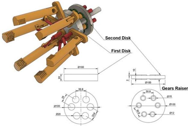
Figure 6. The first and Second Circular Disks
