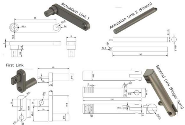
Figure 4. Finger Assembly dimensions in (mm)
