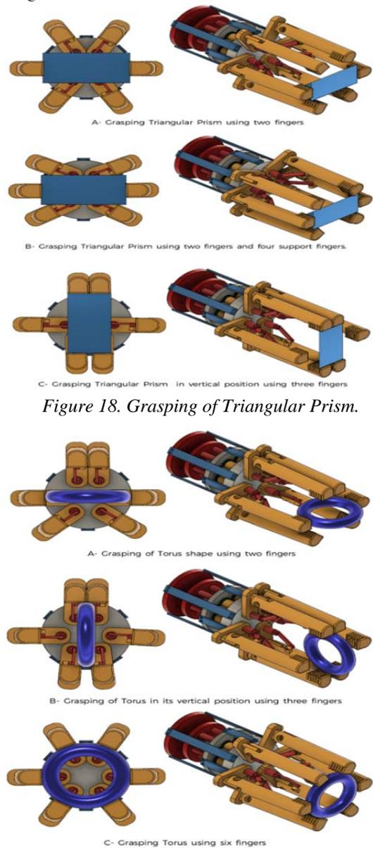
Figure 18. Grasping of Triangular Prism.
