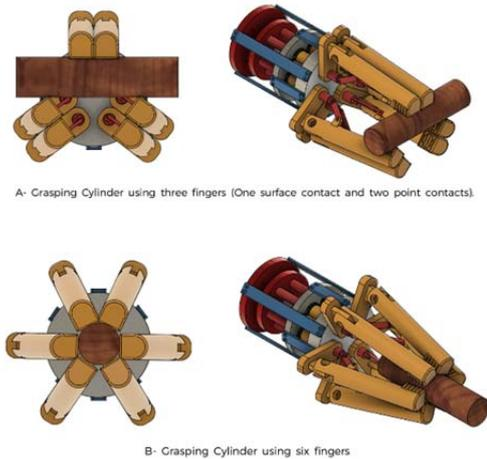
Figure 15. (A)- Grasping Cylinder using three fingers (one surface contact and two-point contacts) (B)- Grasping Cylinder using six fingers
