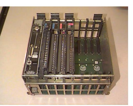
Mini - These are smaller than full sized PLC racks, but can have the same IO capacity.
