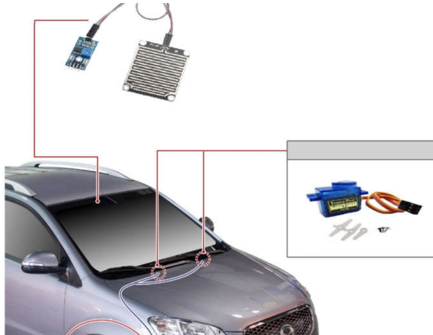
Figure 3.3.1 Exterior view of applied Components (rain sensor and Servo motor)
