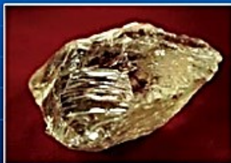
Quartz has a hardness of 7 and shows conchoidal fracture
