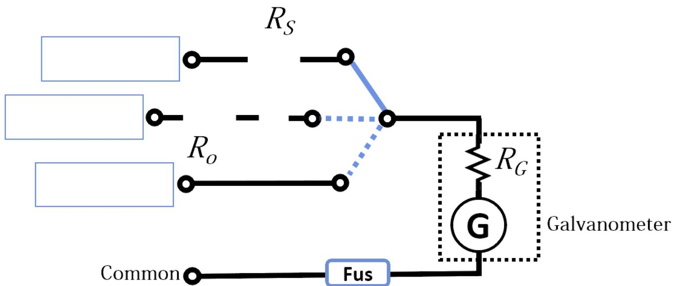
Q2/Write the missing parts of the electric circuit of the shown Multimeter:
