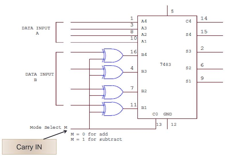
Example: Given the two binary numbers X = 1010100 and Y = 1000011, perform the subtraction (a) X - Y and (b) Y - X using 2's complements
