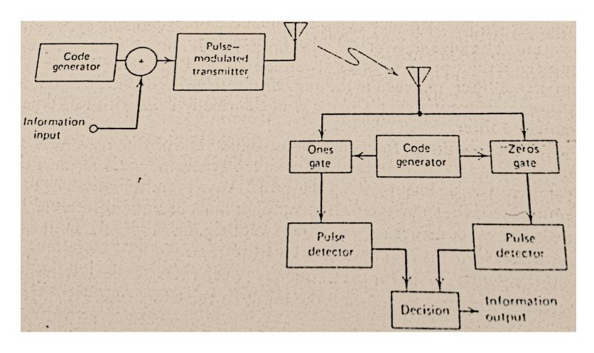
$G_P=1/T_d$ Where  $T_d$  is transmit duty cycle
