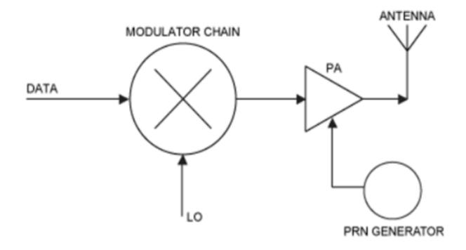
Pulse modulation; PN is used to key the transmitter on-off.
