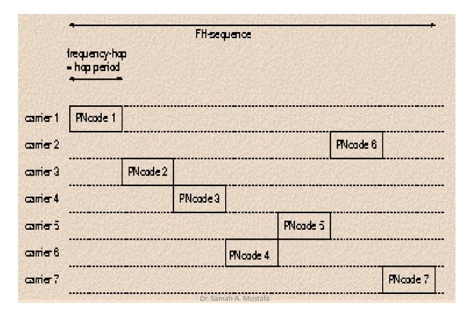
As the FH-sequence and the PN-codes are coupled, an address is a combination of an FH-sequence and PN-codes.
