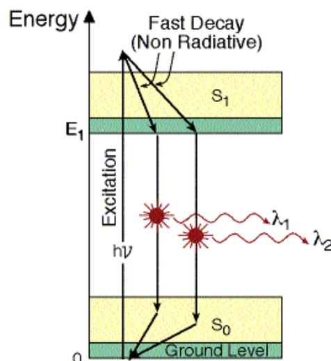
Figure 5.20: Simplified Energy Level Diagram of Dye Laser.
