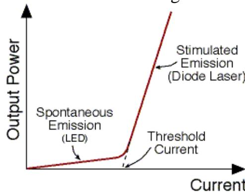
Figure 5.18: Output power from a diode laser as a function of input current.
