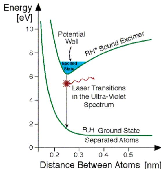
Figure 5.8: Energy levels in the Excimer Laser.
