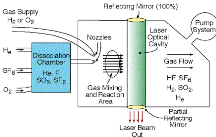
Figure 5.9: The Basic Structure of the Chemical Laser
