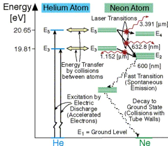
Figure 5.1: Energy Level Diagram of He-Ne Laser
