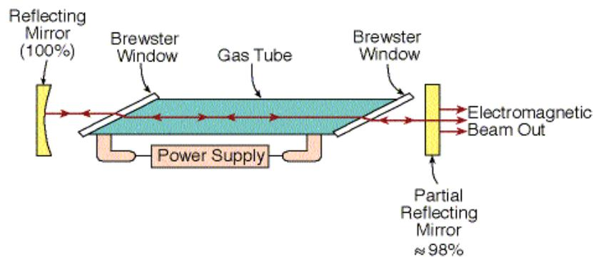
Figure 5.2: The Cavity Structure of He-Ne Laser
