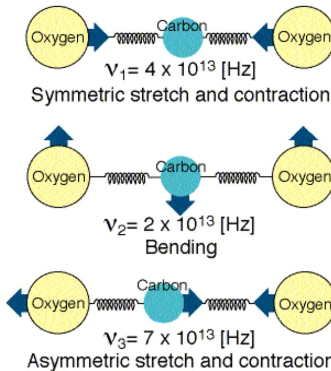
Figure 5.5: Oscillation Modes of CO<sub>2</sub> Molecule
