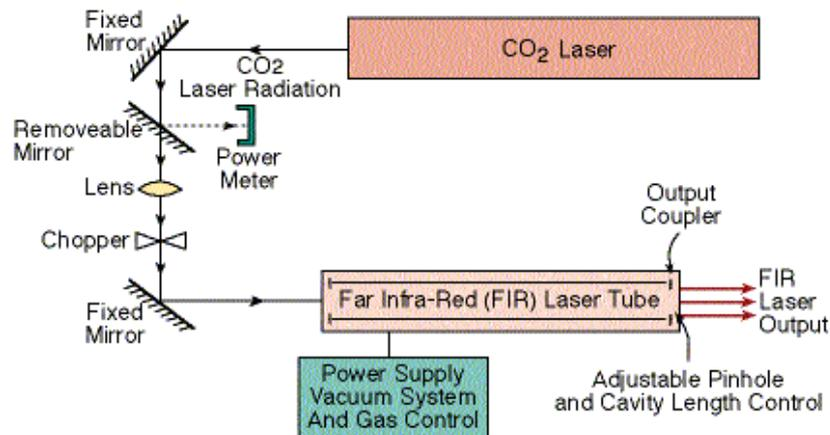
Figure 5.10: schematic drawing of FIR laser
