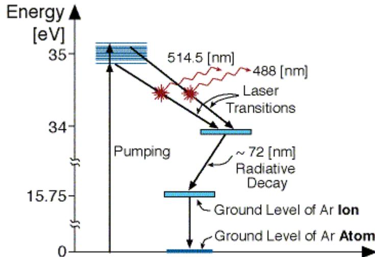
Figure 5.4: Energy Level Diagram of Ion Argon Laser.
