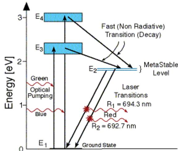
Figure 5.11: Energy Level Diagram of a Ruby Laser
