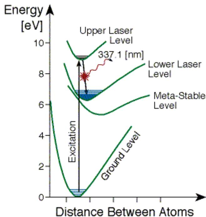
Figure 5.7: Energy level diagram of Nitrogen laser.
