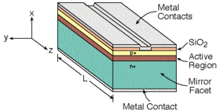
Figure 5.17: Basic structure of a laser diode.
