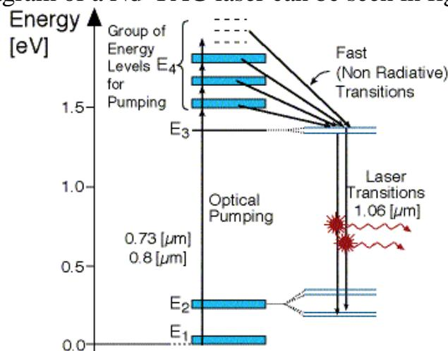
Figure 5.13: Energy Level Diagram of a Nd-YAG Laser
