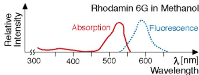
Figure 5.19: Absorption Spectrum (solid line) and Emission Spectrum (dashed line) of Rhodamin 6G in Methanol.
