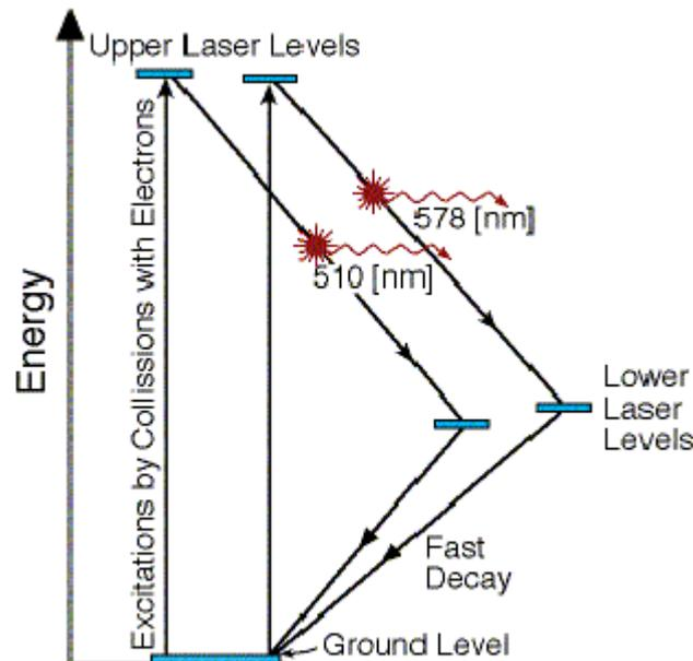
Figure 5.3: Energy Level Diagram of Copper Vapor Laser
