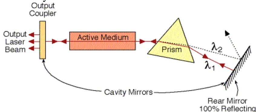
Figure 5.15: Choosing a single wavelength in a tunable laser with a prism.
