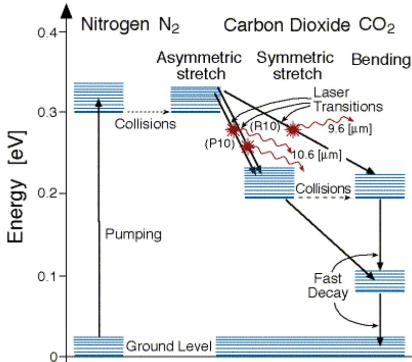
Figure 5.6: Energy Level Diagram of CO<sub>2</sub> Laser
