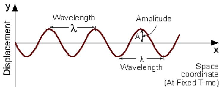
Fig 1.1: Displacement as a function of space coordinates (at fixed time)
