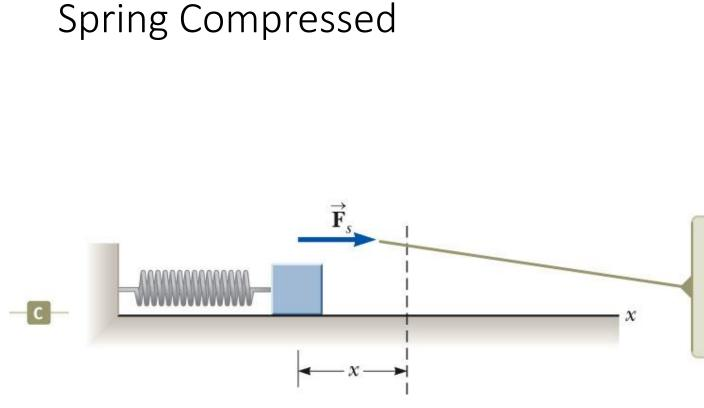
When *x* is negative (compressed spring), the spring force is directed to the right.
