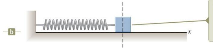
When *x* is zero (natural length of the spring), the spring force is zero.
