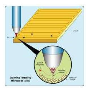
Figure 2.1: Illustrates the idea of scanning tunneling microscope needle work.
