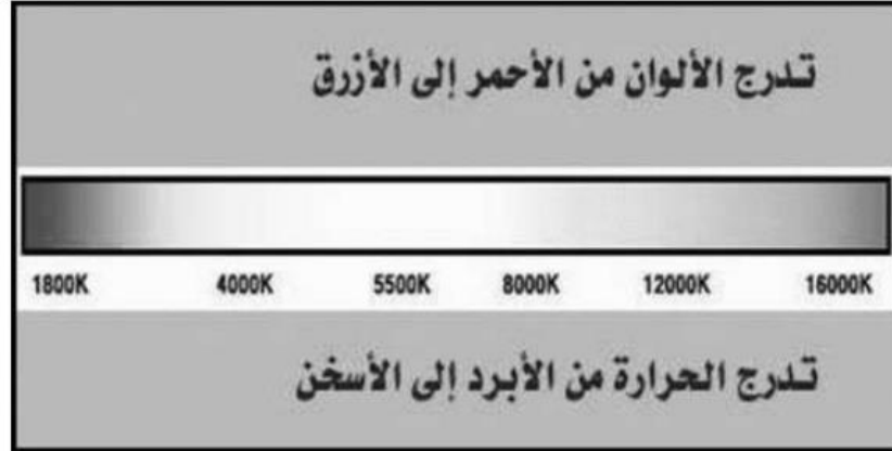
Figure (3-1): Heating any object will give light its colour red at first, and as the body temperature rises, the colour gradients towards light colours until it reaches white, and then as the temperature rises, the colour gradients towards dark colours towards dark blue.[6]
