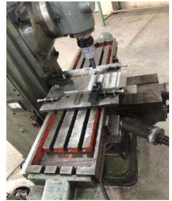
Figure 7 Arrangement of sample and the base on milling machine
