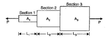
Though each section is subjected to the same axial load P, yet the stress, strains and change in length will be different. The total change in length will be obtained by adding the changes in length of individual section.
