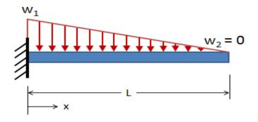
For solving numerical problems, the total load is equal to the area of the triangle and this total load is assumed to be acting at the center of gravity of the triangle at a distance of 2/3 of total length of beam.
