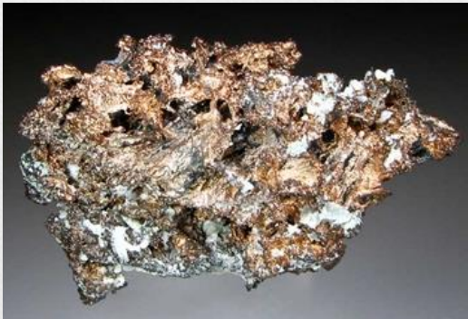
Hackly fracture/ Copper mineral
