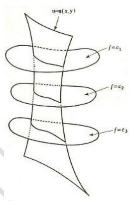
Since both the surfaces intersect orthogonally, at point of intersection (x, y, z) their respective normals are perpendicular.
