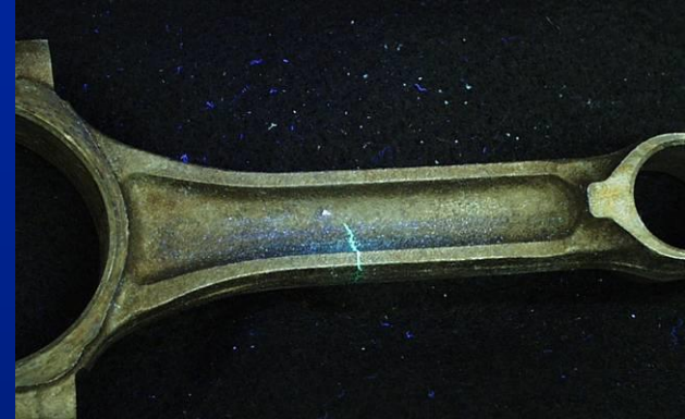
Fluorescent penetrant indication
