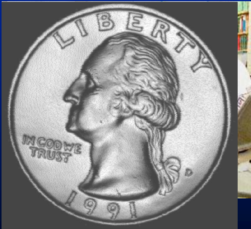
Gray scale image produced using the sound reflected from the front surface of the coin
