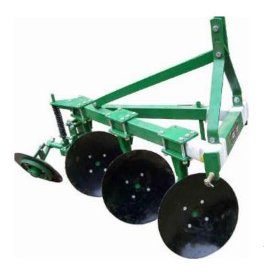
Disc plows cuts in terms soil by using discs instead of a wedge-shaped blade. The idea behind using a disk instead of something like a mold board plow is to help reduce friction. Its sufficient in cases where you have sticky or rocky soil. But its don't do a very good job of covering weeds, so if you're trying to turn over the weeds in moldboard plow is a better choice.
