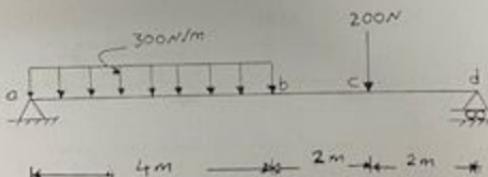
65/ Find the deflection at point ( d ) of the loaded beam as shown in fig. Using double integration method. If  $E = 200 \text{ KN/mm}^2$ ,  $I = 2 \cdot 10^6 \text{ mm}^4$ .
