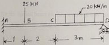
67/ Find the reactions at A and D for the loaded beam as shown in fig. using unit load method. EI = Constant.
