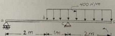
62/ Find the deflection at point D, using unit load method. If  $E = 200 \text{ KN/mm}^2$ ,  $I = 2 \cdot 10^6 \text{ mm}^4$
