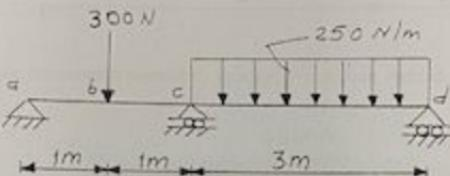
71/ Find the reactions at A & D for the loaded beam as shown . Using unit load method
