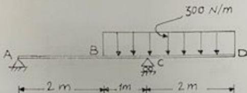
64/ Find the deflection and slope at point C ( $\Delta_c$ ,  $\sigma_c$ ) of the loaded beam as shown in fig. Unit load method. If  $E = 200 \text{ KN/mm}^2$ ,  $I = 1 \cdot 10^6 \text{ mm}^4$ .
