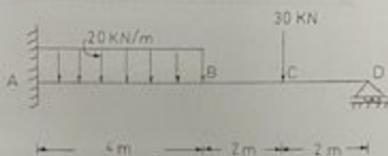
68/ Find the reactions at A , B and D for the loaded beam as shown . Using unit load method , EI = Constant.
