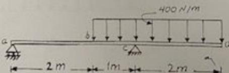
66/ Find the reaction at A and D using unit load method. If EI = Constant
