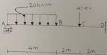
70/ Find the reactions at A , C and D for the loaded beam as shown . Using unit load method.
