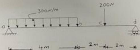
65/ Find the deflection at point ( d ) of the loaded beam as shown in fig . Using double integration method . If  $E = 200 \text{ KN/mm}^2$ ,  $I = 2 \cdot 10^6 \text{ mm}^4$
