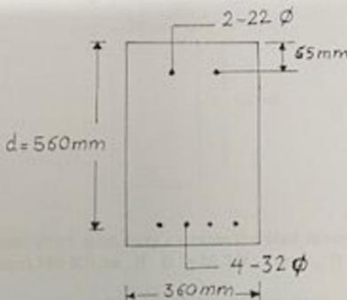
31/ A rectangular beam which must carry a service live load moment 260 KN.m, and dead load moment 190 KN.m. If  $f'_c = 27.6 \text{ N/mm}^2$ ,  $d' = 60 \text{ mm}$ ,  $f_y = 414 \text{ N/mm}^2$ . Find area of the wanted steel (if required compression steel).
