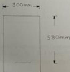
32/ A rectangular beam which must carry a service live load moment 250 KN.m, and dead load moment 200 KN.m. If  $f'_c = 27.6 \text{ N/mm}^2$ ,  $f_y = 414 \text{ N/mm}^2$ . Find area of the wanted steel (if required compression steel),  $d' = 60 \text{ mm}$ .
