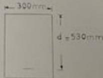
40/ A rectangular beam which must carry a service live load moment 180 KN.m and dead load moment 130 KN.m. If  $f'_c = 20.7 \text{ N/mm}^2$ ,  $f_y = 414 \text{ N/mm}^2$ . Find area of the wanted steel ( If required compression steel ).  $d' = 90 \text{ mm}$
