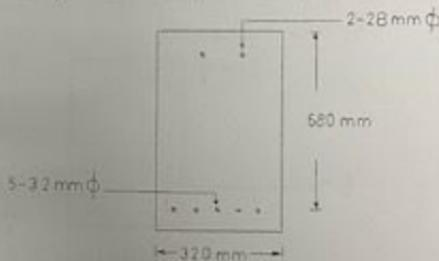
**19/** Find the Ultimate strength ( $M_u$ ) of the beam reinforced section as shown in fig. then check the steel ratio .If  $f'_c = 27.6 \text{ N/mm}^2$ ,  $f_y = 414 \text{ N/mm}^2$ ,  $d' = 70 \text{ mm}$ ,  $E_s = 200.000 \text{ N/mm}^2$ .
