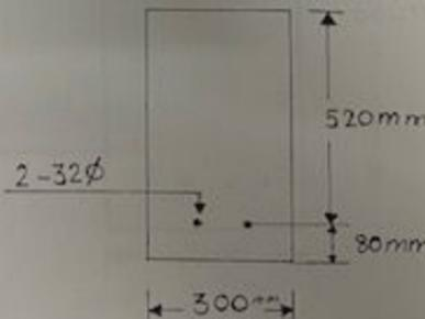
17 / Find the ultimate moment strength ( $M_u$ ) of the beam reinforced section as shown in fig.
