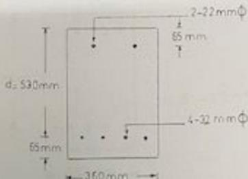
**18/** Determine the Ultimate moment capacity ( $M_u$ ) of the beam reinforced section as shown in fig. If  $f'_c = 27.6 \text{ N/mm}^2$ ,  $f_y = 414 \text{ N/mm}^2$ ,  $d' = 70 \text{ mm}$ ,  $E_s = 200.000 \text{ N/mm}^2$
