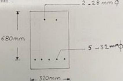
21/ Calculate the Ultimate moment strength ( $M_U$ ) of the beam section as shown in fig. If  $f'_c = 35 \text{ N/mm}^2$ ,  $f_y = 420 \text{ N/mm}^2$ ,  $d' = 65 \text{ mm}$ ,  $E = 200.000 \text{ N/mm}^2$ .
