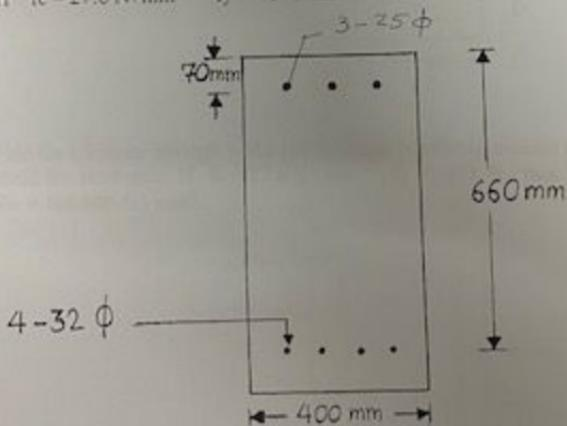
**17/** Find the ultimate moment strength ( $M_u$ ) of the beam reinforced section as shown in fig. If  $f'_c = 35 \text{ N/mm}^2$ ,  $f_y = 420 \text{ N/mm}^2$ ,  $d' = 65 \text{ mm}$ ,  $E_s = 200.000 \text{ N/mm}^2$ .
