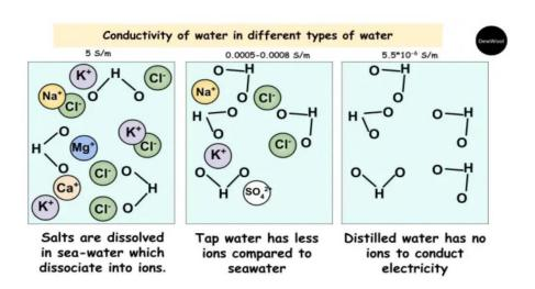
The unit of measurement is **microsiemens per cm** (µS/cm).
