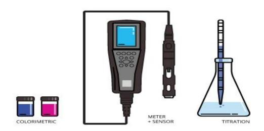
Dissolved oxygen can be measured by colorimetry, a sensor and meter or by titration
