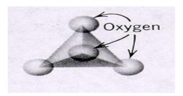
2-phylosilicates:- continuous sheets the tetrahedral sheet each sharing three oxgyens Si:O ratio 2:5  $[Si_2O_5]^{2-}$  such as mica and montmorillonite
