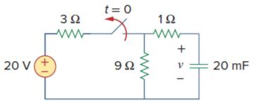
**Q48**) The switch in figure below has been in position A for a long time. At t = 0, the switch moves to **B**. Determine v(t) for t > 0 and calculate its value at t = 1 and 4 s.
