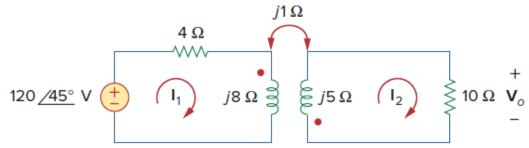
**Q6**) Determine the phasor currents  $I_1$  and  $I_2$  in the circuit shown in figure below.
