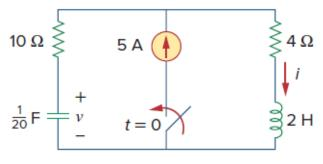
**Q89**) Find  $v_o(t)$  for t > 0 in the circuit of figure below.
