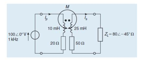
**Q19**) For the magnetically coupled circuit shown in figure below. Determine (a) the source current and (b) the load current. (c) If one of the windings is reversed, determine the new value of source and load currents.
