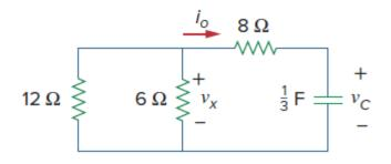
**Q55**) If the switch in Figure below opens at t = 0, find v(t) for  $t \ge 0$  and  $w_C(0)$ .
