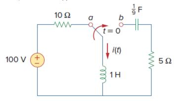
**Q84**) Refer to the circuit shown in figure below Find v(t) for t > 0.
