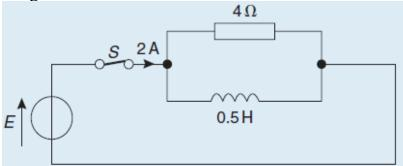
**Q74**) For the circuit in figure below, find i(t) for t > 0.
