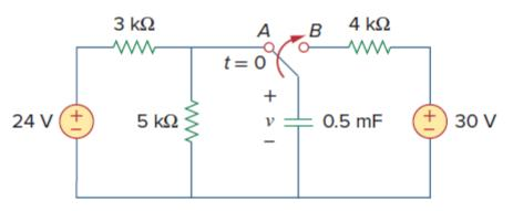
**Q49**) In figure below, the switch has been closed for a long time and is opened at t = 0. Find *i* and *v* for all time.
