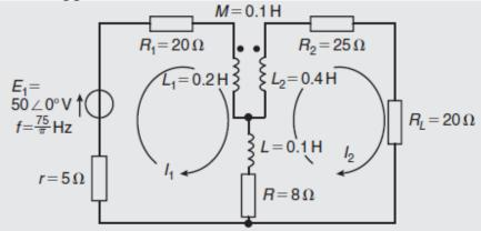
**Q15**) For the magnetically coupled circuit shown in figure below, determine (a) the self impedance of the primary circuit, (b) the self impedance of the secondary circuit, (c) the primary current and (d) the secondary current.
