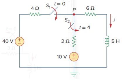
**Q67**) Find i(t) in the circuit of figure below for t > 0. Assume that the switch has been closed for a long time.
