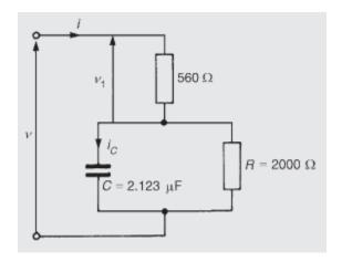
Q28) A voltage waveform having a fundamental of maximum value 400 V and a third harmonic of maximum value 10 V is applied to the circuit shown in figure below. Determine (a) the fundamental frequency for resonance with the third harmonic, and (b) the maximum value of the fundamental and third harmonic components of current.
