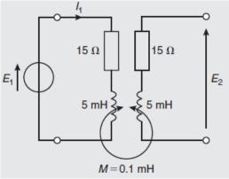
Q10) For the circuit shown in figure below, determine the value of the secondary current  $I_2$  if  $E1 = 2 \angle 0^\circ$  volts and the frequency is  $10^{^3}/\pi$  Hz.
