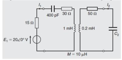
Q12) For the coupled circuit shown in figure below, determine the values of currents  $I_1$  and  $I_2$ .
