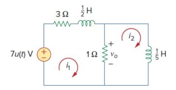
**Q90**) For t > 0, obtain  $v_o(t)$  in the circuit of figure below (*Hint:* First find  $v_1$  and  $v_2$ .)
