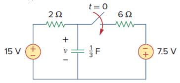
Q57) The switch in figure below is closed at t = 0. Find i(t) and v(t) for all time. Note that u(-t) = 1 for t < 0 and 0 for t > 0. Also, u(-t) = 1 - u(t).
