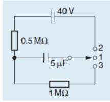
**Q54**) For the circuit in figure below. Let  $v_c(0) = 60$  V. Determine  $v_c$ ,  $v_x$ , and  $i_o$  for  $t \ge 0$ .
