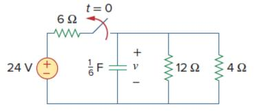
**Q56**) Find v(t) for t > 0 in the circuit of Figure below. Assume the switch has been open for a long time and is closed at t = 0. Calculate v(t) at t = 0.5.
