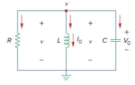
**Q81**) Find v(t) for t > 0 in the *RLC* circuit of figure below.
