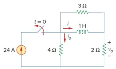
**Q76**) The switch in figure below has been closed for a long time. It opens at t = 0. Find i(t) for t > 0.
