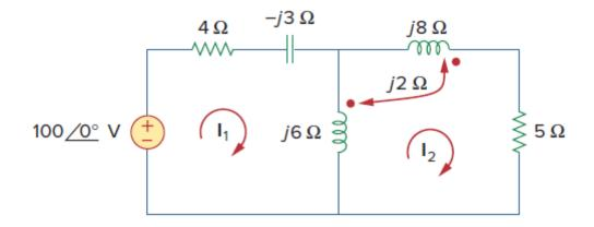
Q3) Consider the circuit shown in figure below. Determine the coupling coefficient. Calculate the energy stored in the coupled inductors at time t = 1s if  $v = 60 \cos (4t + 30^\circ) V$ .
