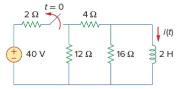
**Q65**) In the circuit shown in figure below, find  $i_o$ ,  $v_o$ , and i for all time, assuming that the switch was open for a long time.
