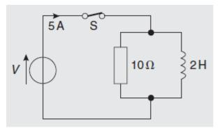
**Q64**) The switch in the circuit of figure below has been closed for a long time. At t = 0, the switch is opened. Calculate i(t) for t > 0.
