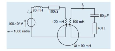
**Q16**) In the coupled circuit shown in figure below, each winding is tuned to resonance at the same frequency. Calculate (a) the resonant frequency, (b) the value of CS, (c) the primary current, (d) the secondary current, (e) the voltage across capacitor CS and (f) the coefficient of coupling.
