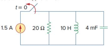
**Q85**) Having been in position *a* for a long time, the switch in figure below is moved to position *b* at t = 0. Find v(t) and  $v_R(t)$  for t > 0.
