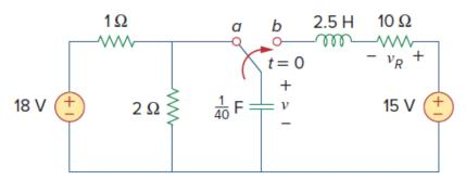
**Q86**) Find i(t) and v(t) for t > 0 in the circuit of figure below.
