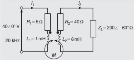
**Q14**) For the coupled circuit shown in figure below. Determine the source and load currents for (a) the windings as shown (i.e. with the dots adjacent), and (b) with one winding reversed (i.e. with the dots at opposite ends).
