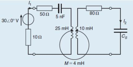
**Q17**) Determine the values of currents  $I_p$  and  $I_s$  in the coupled circuit shown in figure below.
