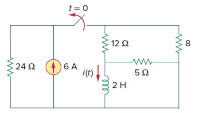
**Q75**) Determine i,  $i_o$ , and  $v_o$  for all t in the circuit shown in figure below. Assume that the switch was closed for a long time. It should be noted that opening a switch in series with an ideal current source creates an infinite voltage at the current source terminals. Clearly
