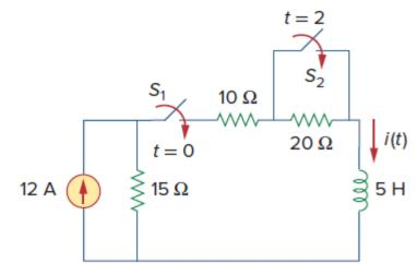
**Q78**) Find i(t) in the circuit of figure below. Assume that the circuit has reached steady state at  $t = 0^{-1}$ .
