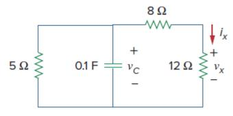
Q47) The switch in the circuit in figure below has been closed for a long time, and it is opened at t = 0. Find v(t) for  $t \ge 0$ . Calculate the initial energy stored in the capacitor.
