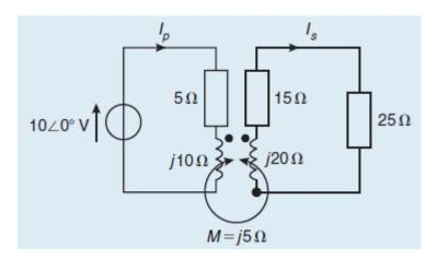
**Q18**) The **coefficient of coupling** between the primary and secondary windings for the air-cored transformer shown in figure below is 0.84. Calculate for the circuit (a) the mutual inductance M, (b) the primary current  $I_p$  and (c) the secondary current  $I_s$ .
