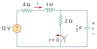
**Q88**) Determine v and i for t > 0 in the circuit of figure below.
