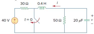
**Q82**) In the circuit of figure below, find i(t) and  $i_R(t)$  for t > 0.
