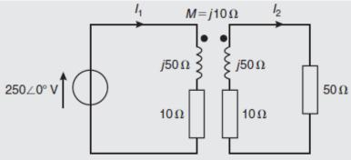
Q13) The circuit diagram of an air-cored transformer winding is shown in figure below. The coefficient of coupling between primary and secondary windings is 0.70. Determine for the circuit (a) the mutual inductance M, (b) the primary current  $I_1$  and (c) the secondary current  $I_2$ .
