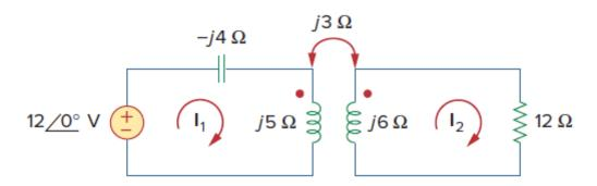
Q2) Calculate the mesh currents in the circuit shown in figure below.
