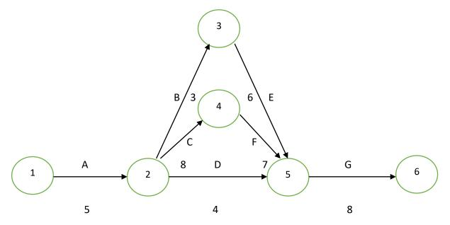
Consider the paths, beginning with the start node and stopping with the end node. There are three such paths for the given project. They are as follows:
