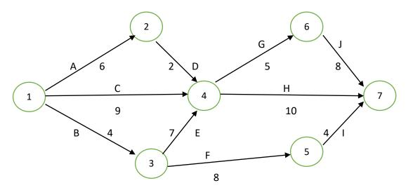
Consider the paths, beginning with the start node and stopping with the end node. There are three such paths for the given project. They are as follows:
