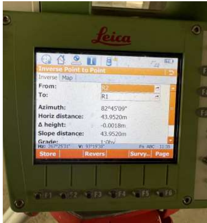
Figure 3-2: Establishing reference line on total station
