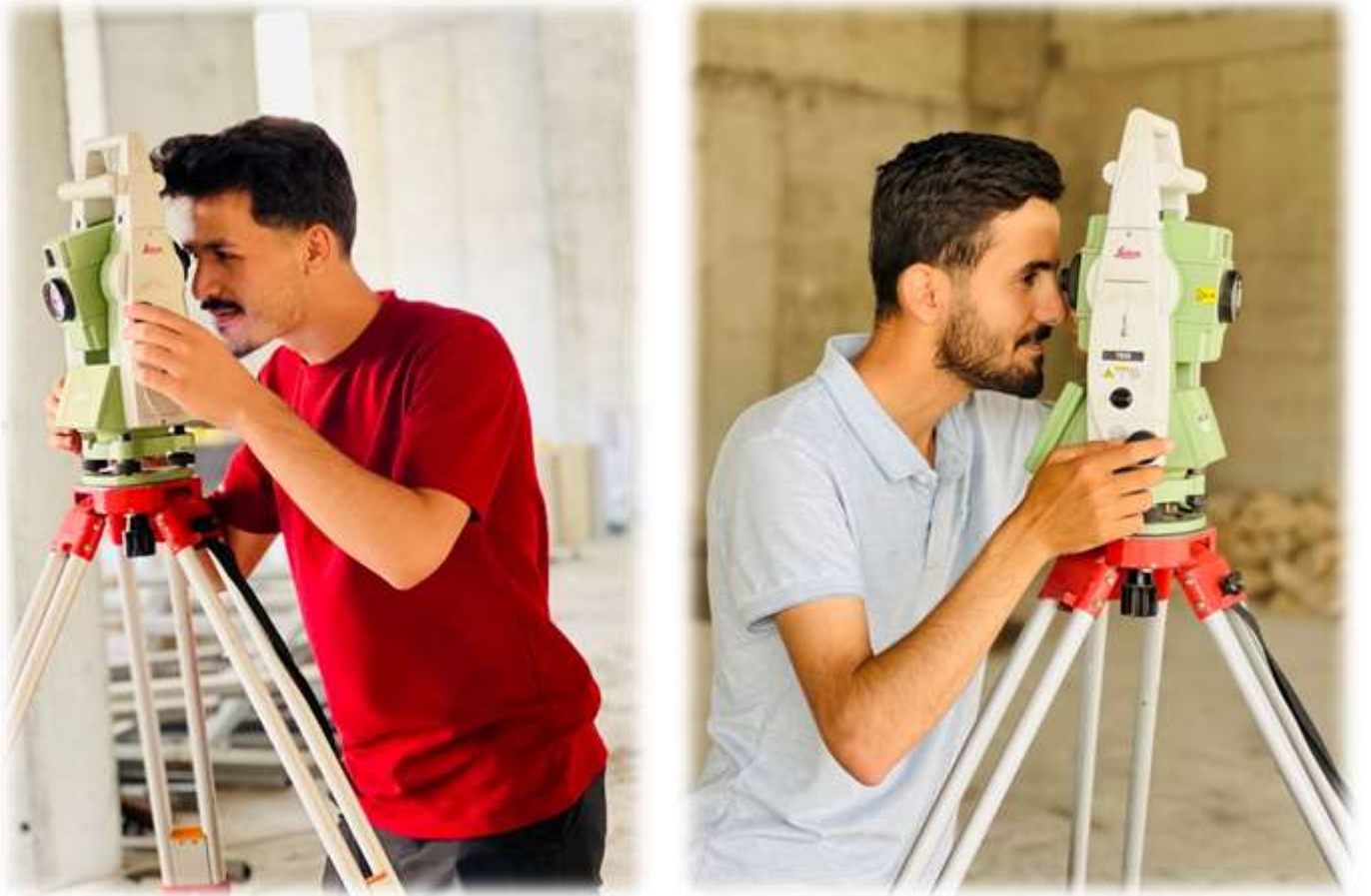
Figure 3-15: While collecting data by Leica TS15 total station
