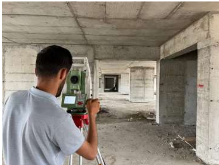
Figure 3-7: Measure points using total station Leica TS15
