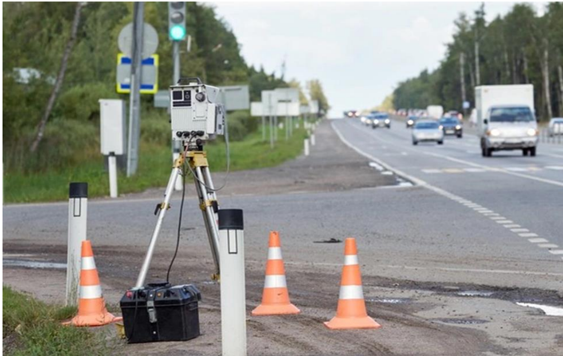
Fig.(4) We use radar to detect cars going faster than the speed limit.
