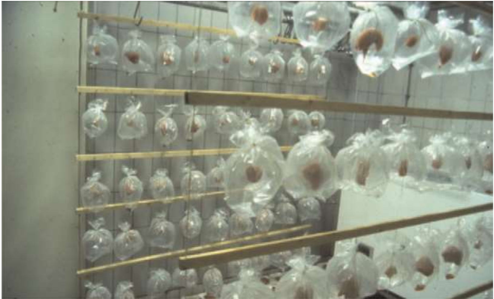
Figure Image of the gravimetric method for measuring drip loss, involving suspension of a meat sample in an inflated bag and storage at 2–4 °C for 1–2 days.
