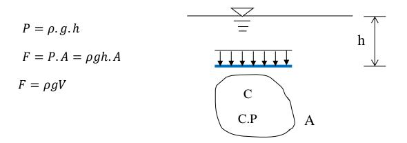
The resultant force F passes through a point on the plane surface defined as the center of pressure (CP), for a horizontal plane CP will coincide with the centroid (C) of the surface.
