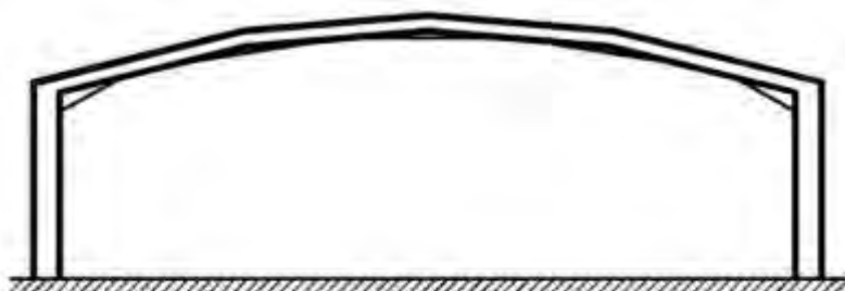
(c) Mansard portal (spans up to 60 m)
