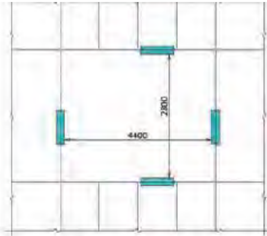
FRAMED OPENING FOR STAIRS
