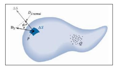
The electric flux density  $D_S$ At P due to Charge Q. The total flux passing through  $\Delta S$  is  $\Delta D_S \cdot \Delta S$ .
