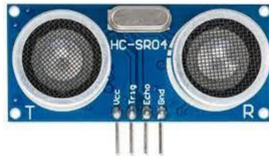
Fig. 3. Ultrasonic sensor for ultrasonic wave production in motion detection.
