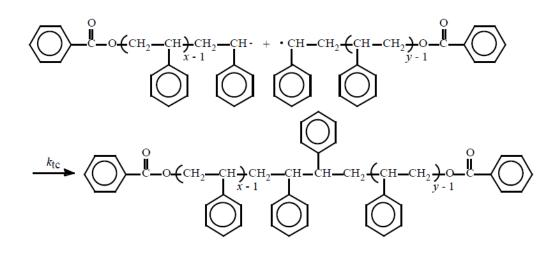
The above structure shows a single head-to-head placement of styrene units at the combination site.
