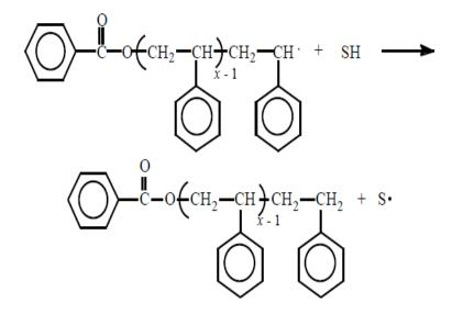
As illustrated, the radical site is transferred to the chain-transfer agent (S  $\cdot$ ), which can then a d d monomer units to continue the polymerization process. Subsequent termination of the growing chain-transfer radical chain (SM<sub>x</sub> $\cdot$ ) will result in a terminated chain having one (i.e., termination by disproportionation) or two (i.e., termination by combination) chaintransfer (S) groups at the polymer ends.
