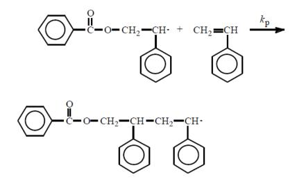
Additional monomers are a d d e d sequentially during subsequent propagation steps, as represented by the generalized equation
