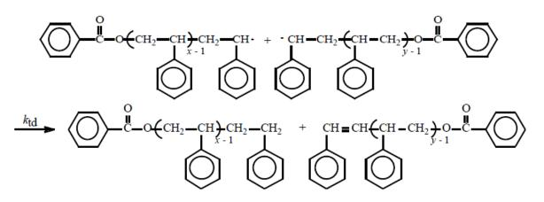
In addition to termination by combination and disproportionation, another mechanism of termination is *chain transfer* by hydrogen abstraction from an initiator, monomer, polymer, or solvent molecule. In general terms, this process may be represented as
