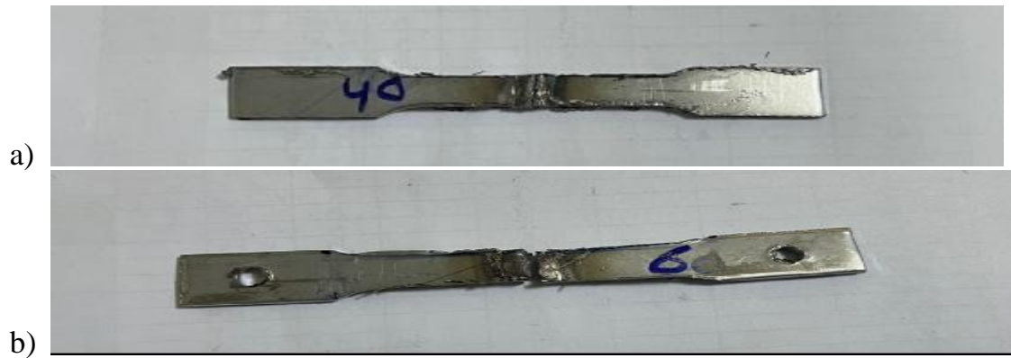
Figure 3.6 Experiment result of Tensile testing. a) 40s; b) 60s.
