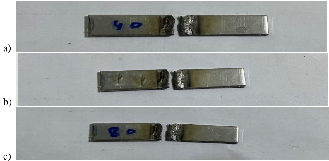
Figure 3.4 Experiment result of Impact testing. a) 40s; b) 60s; c) 80s.
