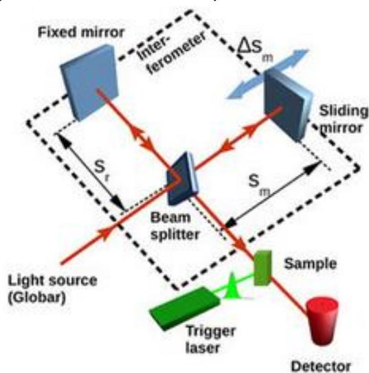
Globar is silicon carbide rod 20-50 mm and width 5-10 mm it is heated to temperatures of 1000 to 1650°C in the near infrared range. They produce wavelength range from 1 to 50  $\mu\text{m}$ . A Globar source is then combined with an interference filter to produce radiation having wavelengths of 4 to 15  $\mu\text{m}$ .
