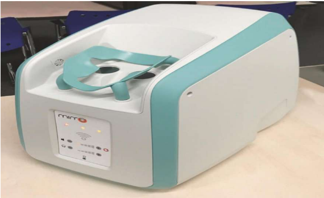
Fig. 2.6 Home-based MIMO-OCT system. Images courtesy of Dr Peter Maloca, University of Basel.
