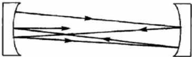
A ray is always reflected back toward the center by the curved mirrors of a stable resonator.
