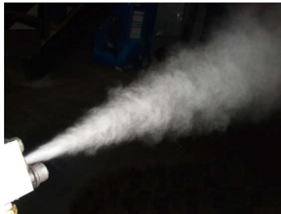
Figure 3. Spraying water into the air inlet manifold.
