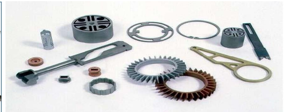
Figure: Difficult internal parts made by EDM process
