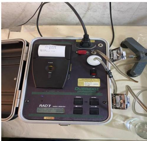
**Fig 2.** Radon detection device (RAD7)
