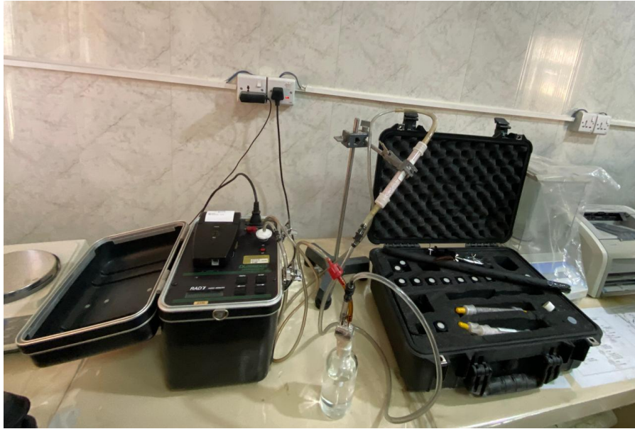
Fig 3. Schematic representation of Radon on water concentration experimental setup.
