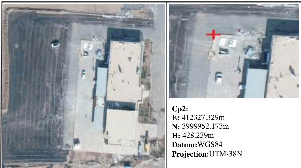
Figure 2.3.2: Location of GCP2-Corner of Concrete
