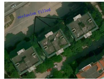
True Orthophoto produced by removing relief displacement by applying the vector data
