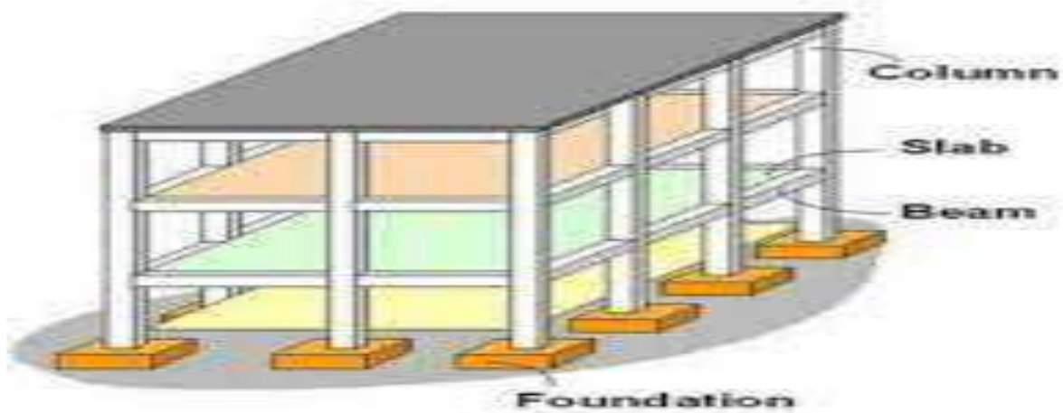
Figure 1-11 Typical R.C. Frame Building
