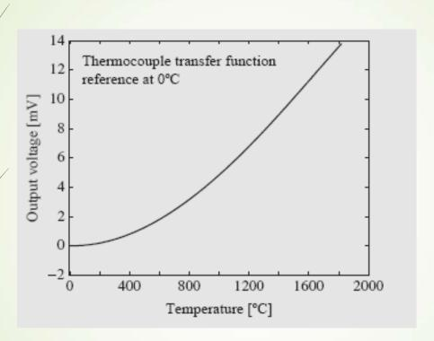
For example, the output of a thermocouple is typically 10–50 µV/C, whereas a piezoelectric sensor can produce 300 V or more in response to motion. A magnetic actuator may require, say, 20 A at 12 V, whereas an electrostatic actuator may operate at 500 V (or higher) at a very low current.
