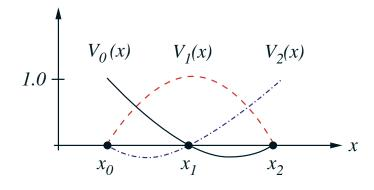
• Note that the location of the roots of  $V_0(x)$ ,  $V_1(x)$  and  $V_2(x)$  are defined such that the basic premise of interpolation is satisfied, namely that  $g(x_i) = f_i$ . Thus:
