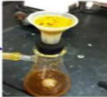
The product was then collected with a Buchner funnel and washed with cold water.
