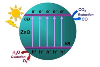
Figure 4: Schematic diagram of CO<sub>2</sub> photoreduction mechanism of ZnO NPs (Liu et al., 2016)
