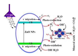
Figure 2: Schematic representation of photocatalytic degradation using ZnO nanoparticles (Alshehri & Malik, 2019)
