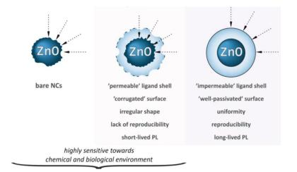
Figure 6: Schematic representation of nanocrystal-ligand interface structure of ZnO NPs (Wolska-Pietkiewicz et al., 2019)
